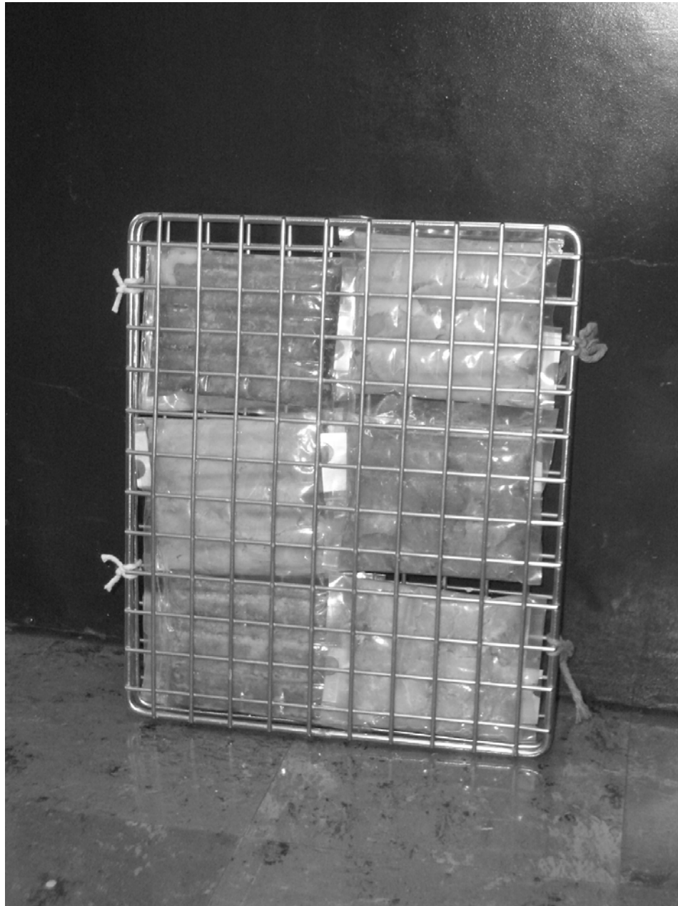
Figure 1.1 SIX RETORTABLE HAM POUCHES IN A 35.5CM X 30.5 CM STAINLESS STEEL MOLD
